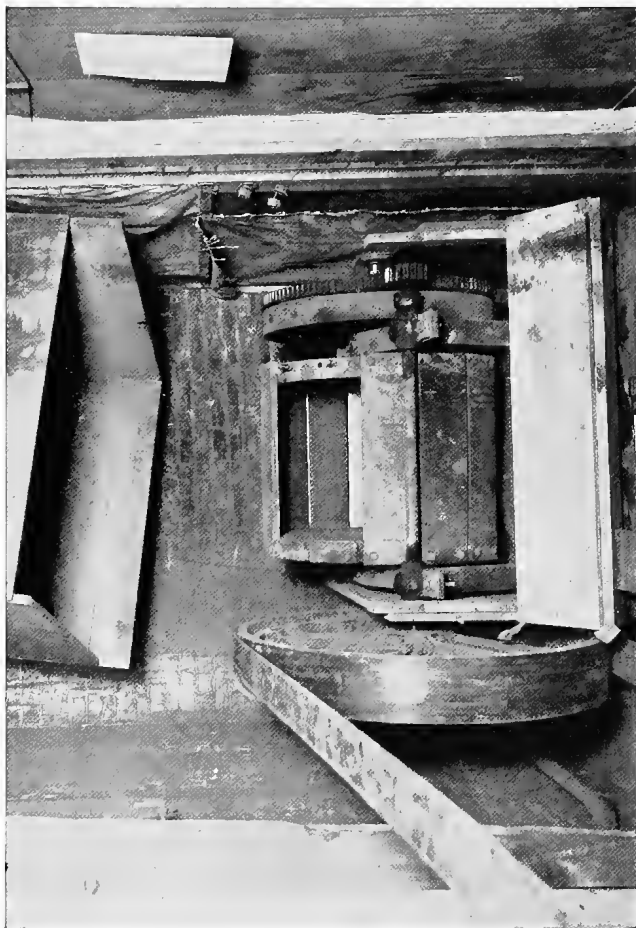
Highway Division, Maryland Geological Survey, 1902. ABRASION AND IMPACT TEST OF PAVING-BRICKS. Standard Machine of 1900.
